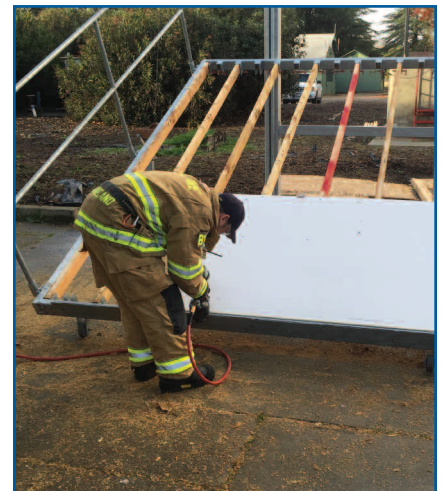
With new sheetrock or plywood the prop is easily prepared for a new training evolution.
